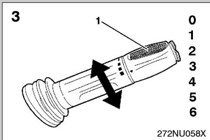
**Engine braking control - Vehicles with intarder**
