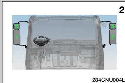
Press the mirror heater button (Fig. 1, ref. 3) to rapidly demist the mirrors. Press the button to turn the mirror heating system on. Press the button again to turn the mirror heating system off.
