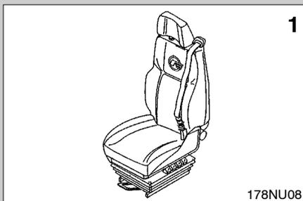
The belt does not need to be adjusted by hand: the webbing adjusts itself automatically to the length most suited to the driver allowing him freedom of movement provided that his movements are not abrupt.
