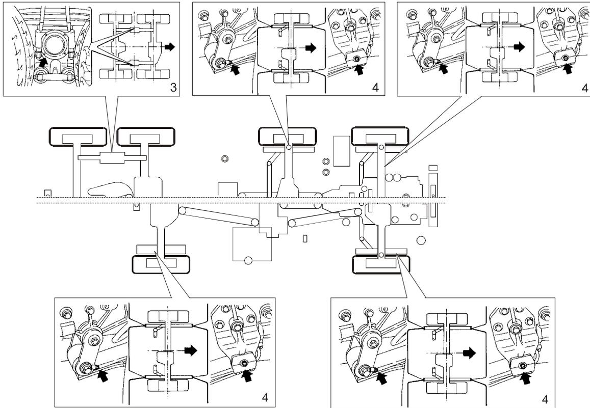
**LOCATION OF COMPONENTS****Suspension greasing****Key (see diagram on previous page)**
