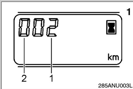
The selected mirror is identified by the number on the LCD (Fig. 1, ref. 1)
