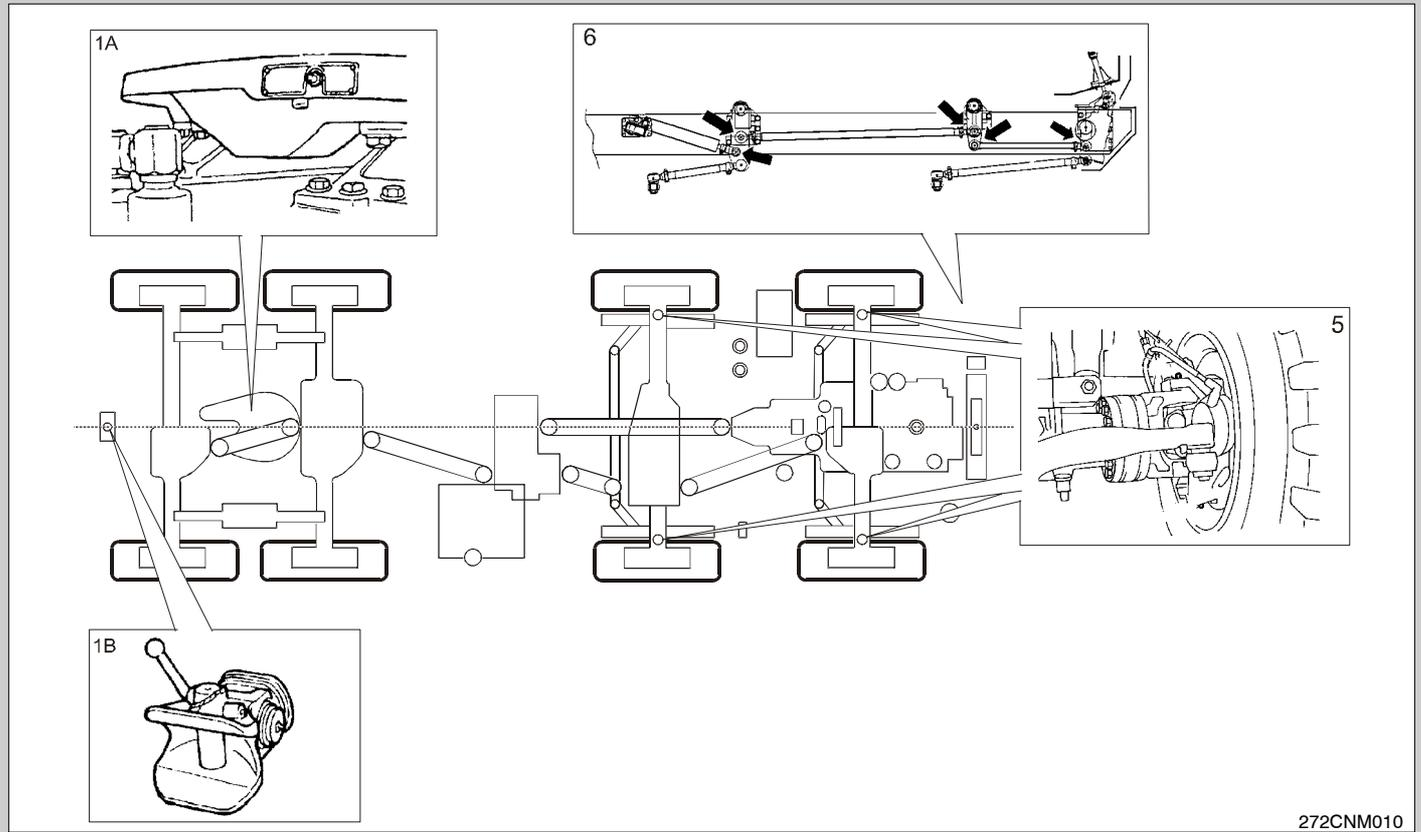
**LOCATION OF COMPONENTS****Steering linkages, semi-trailer fifth wheel, tow hook greasing****Key (see diagram on previous page)**
