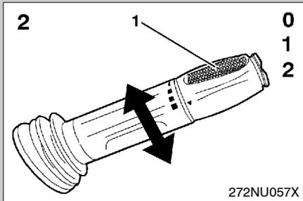
**Engine braking control - Vehicles without intarder**
