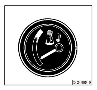
● The needle of the temperature display should always be in the green area, and only as an exception in the yellow/green area. If the needle rises into the orange area the engine is getting too hot. Switch off the engine and determine the cause as per fault table (see 7.1).
