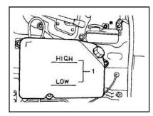
Check reservoir tank for the coolant level. The coolant level should be with in the range 1 shown in the illustration. If the level is low, add coolant by reference to "Replacement of coolant".
