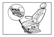
Seat Cushion Height Fixing (Driver's side only) (If installed)
