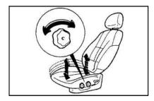
Seat Cushion Height Adjustment (If installed) (Driver's seat only)
