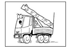
When long cargos are to be loaded, use rigid frames to minimize their protrusion from the rear end of the body.
