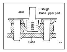
How to adjust inside diameter of jaw
