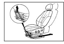
Adjusting Seat Forward and Rearward (If installed)(Driver's side only)
