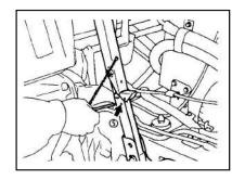
5. Push the cab all the way up, and the cab will be automatically held in position by the cab stay. Insert the safety pin⑤.
