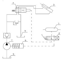
1.Air chamber 5.Fule tank 2.Pneumatic control vavle 6.Cylinder of the power take 7.Gear pump (with an inverted vavle)
