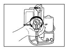
1. Unlock the knob by turning the electric tilting cab key
