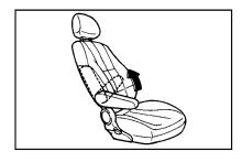
Adjusting Armrest Angle (Driver's side only) (If installed)
