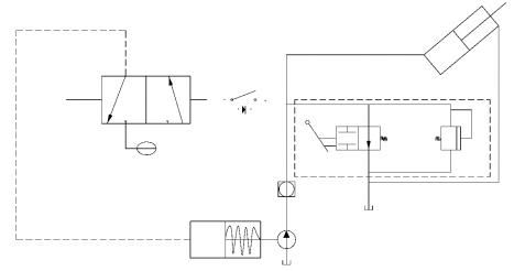
1.Hydraulic cylinder 2.Turning valve (with the relief valve) 3.Fuel tank
