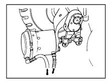
8. Measure the stroke made by the push red of the brake chamber when the brake pedal is depressed all the way. Verify that the stroke is up to specifications given in the following table if it is out of specification, adjust with the worm shaft.
