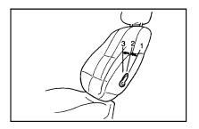
Lumbar Support Adjustment (If installed) (Driver's seat only)
