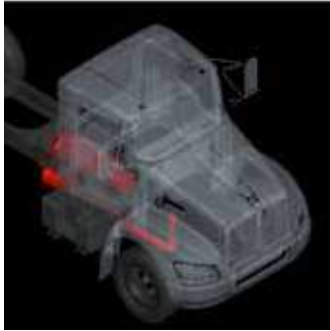
Horizontal DPF and SCR with Horizontal Tailpipe
