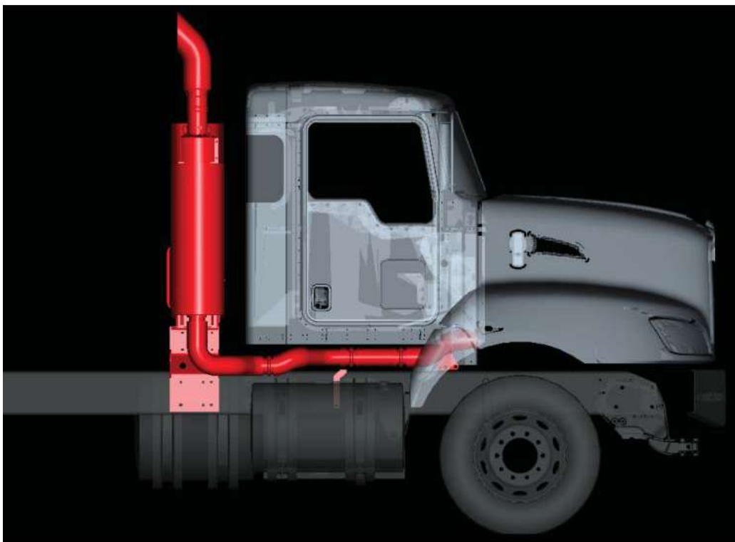
FIGURE 4-20: Right View of Vertical DPF and SCR
