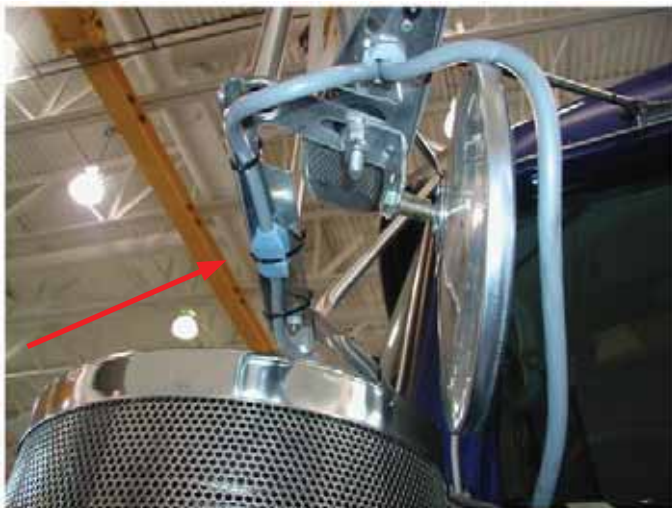
FIGURE 2-3: West Coast Mirror OAT sensor, located in overmold on mirror harness.
