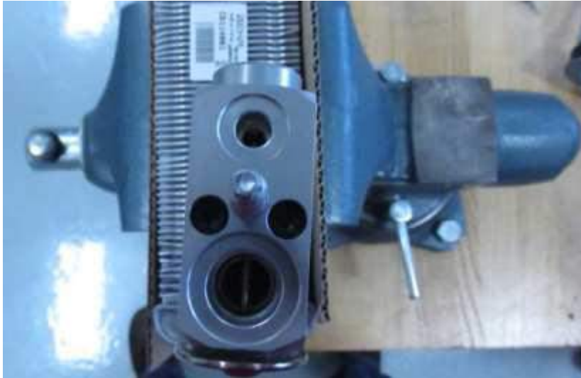
Bench Top Vice With Evaporator Secured
