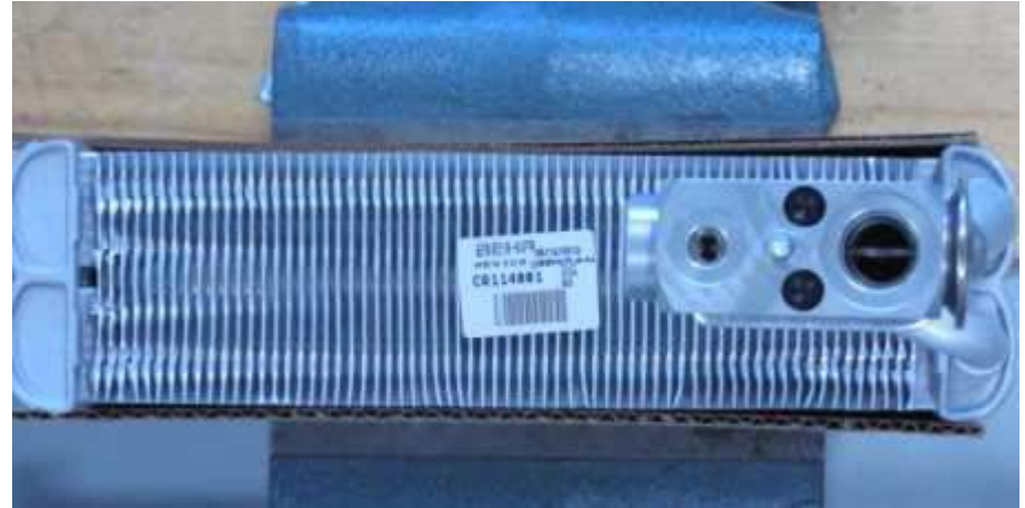
Starting Position of TXV Relative to Evaporator Before Torque Applied
