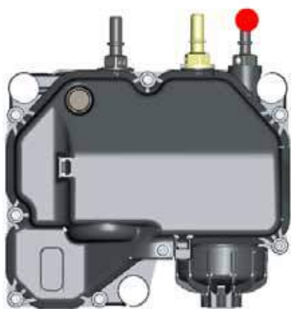
FIGURE 4-1: Measurement Location of DEF Supply Module (Pump)
