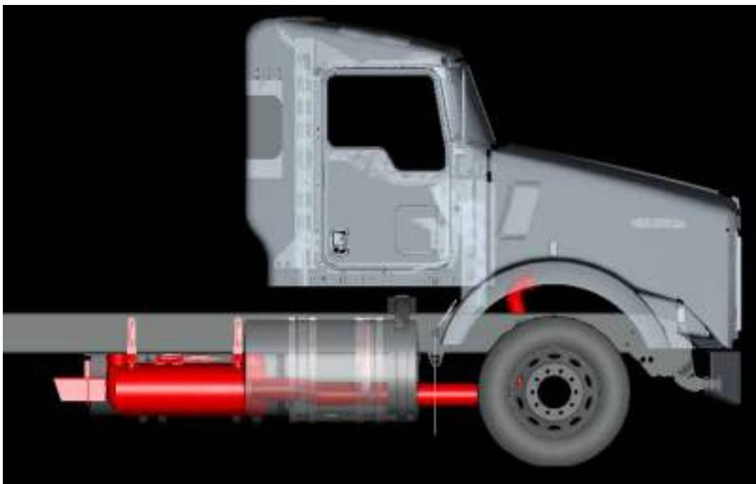
FIGURE 4-29: Right View of Horizontal DPF and SCR with Horizontal Tailpipe
