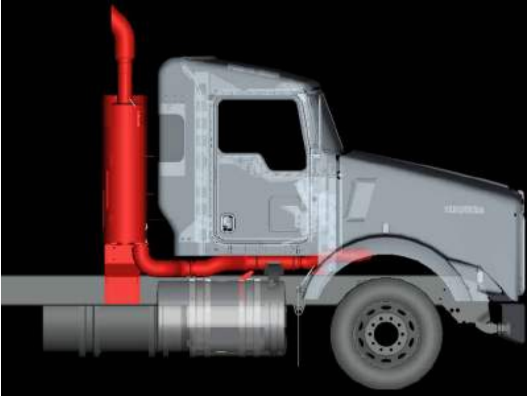
FIGURE 4-33: Right View of Vertical DPF and SCR
