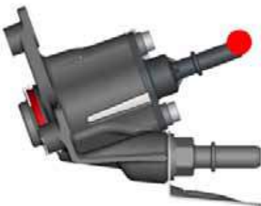
FIGURE 4-2: Measurement Location of DEF Dosing Module (Injector)
