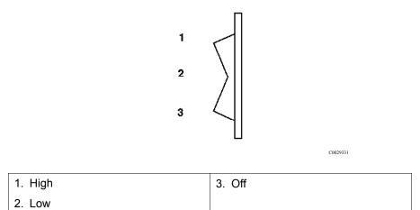
As grades and vehicle weight increase, it will be necessary to use the HIGH position.
