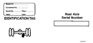
The **MERITOR carrier assembly** serial number is located on the left side of the forward carrier, and the top of the rear carrier.
