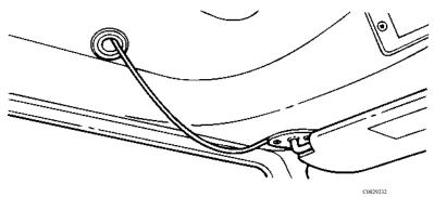
The air horn(s), if equipped, is activated by pulling down on the cord that is located above the driver near the overhead console.
