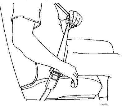
3. To tighten the lap portion of the combination belt, pull upward on the shoulder portion until the lap portion fits snugly. The belt should rest as low on your hips as possible.
