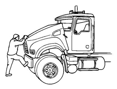
4. Using the Bulldog as a handle, pull on the hood to raise it over the engine. You may put one foot on the bumper if necessary.
