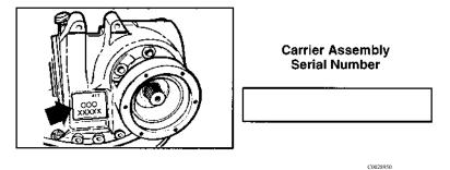
The **Eaton® Spicer® rear axle** serial number is located on the rear of the axle housing toward the carrier.
