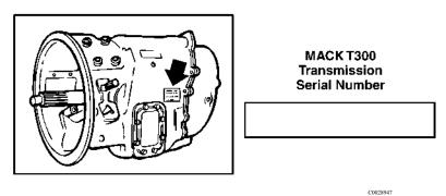
All **Eaton® Fuller® transmission** identification plates are located on the front left side of the main case.
