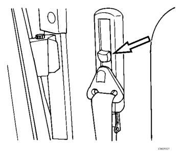
The shoulder belt portion of the three-point belt is adjustable so that the belt can be adjusted to lay properly and comfortably across the shoulder. To adjust the belt, squeeze the release lock and move the belt to the desired position. The belt locks into place when the lock is released.
