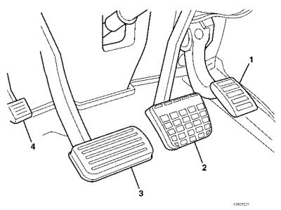
**1. Accelerator Pedal** — Depress to increase engine/vehicle speed; release to decrease engine/vehicle speed.
