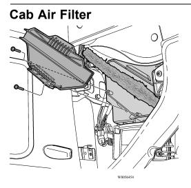
To provide comfortable and clean fresh air in the cab, the heating and air conditioning system is designed with a replaceable filter.
