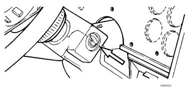
This switch starts the engine (turn the switch clockwise) and activates the accessory relay (turn the switch counterclockwise). When the switch is turned ON (in a clockwise direction), a warning buzzer sounds if air system pressure is below  $448 \pm 34$  kPa ( $65 \pm 5$  psi) or if there is low oil pressure. The buzzer shuts off as soon as sufficient air/oil pressure is restored.
