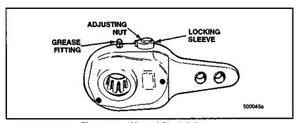
Figure 75 — Manual Slack Adjuster
