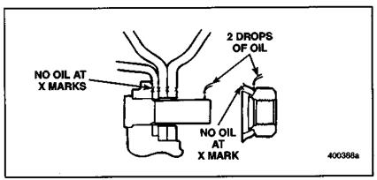
Figure 68 --- Flanged Nut Installation
