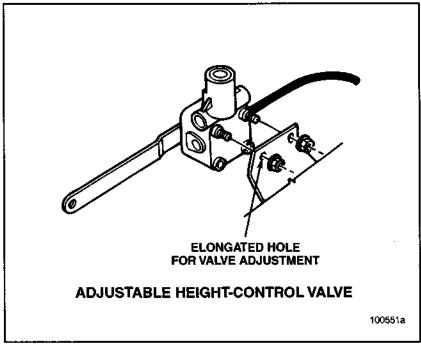
Figure 62 — Adjustable Height Control Valve
