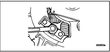
Figure 79 — Adjusting Release Bearing Travel
