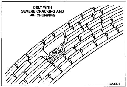
Figure 14 — Belt with Severe Cracking and Rib Chunking
