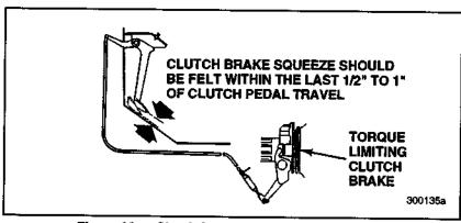
Figure 86 — Clutch Brake Squeeze — Spicer Solo
