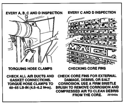
Figure 23 — Charge Air Cooler Maintenance
