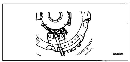
Figure 78 — Release Bearing Adjustment
