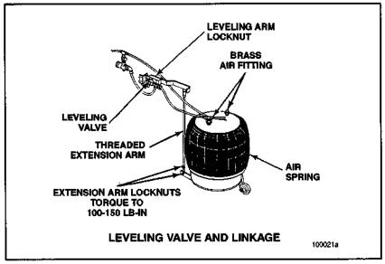
Figure 60 — Height Control Valve and Linkage
