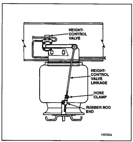
Figure 59 — Leveling Valve and Linkage
