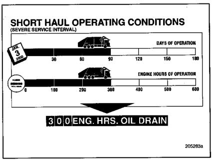
Figure 6 -- Short Haul Operating Conditions
