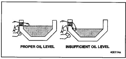
Figure 36 — Oil Level Check
