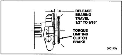
Figure 77 — Release Bearing Travel
