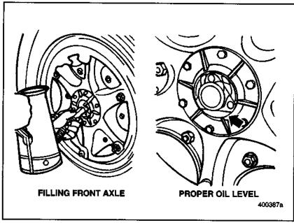
Figure 48 — Front Axle Hub
