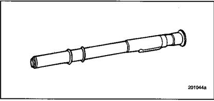
Figure 11 — Tensioning Tool J42185
