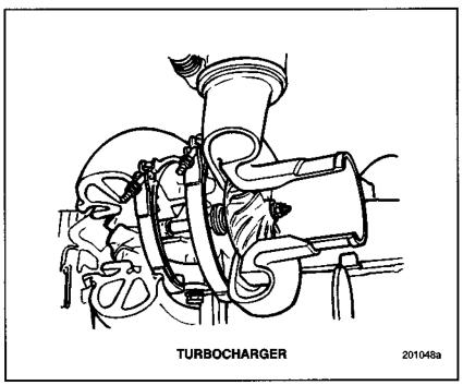
Figure 22 — Turbocharger
