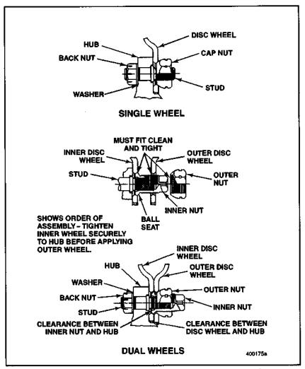
Figure 69 — Disc Wheel Assembly — Stud Located Ball Seat
