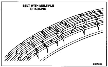
Figure 13 — Belt with Multiple Cracking
