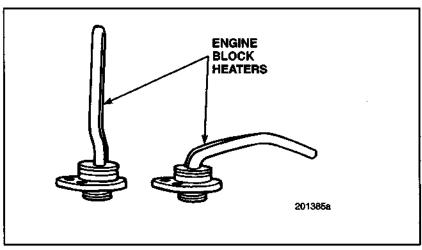
Figure 95 — Engine Block Heaters
