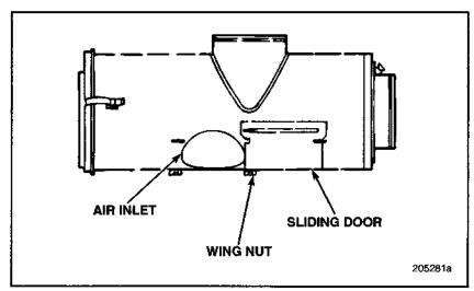
Figure 18 — Dual-Inlet Air Cleaner
