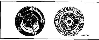
Figure 66 — Spoke Wheel Nut Tightening Sequence
