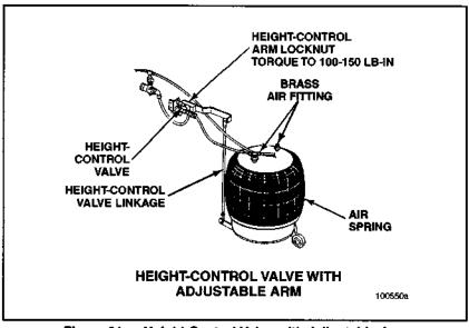
Figure 61 — Height Control Valve with Adjustable Arm
