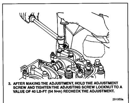
Figure 93 — Valve Lash Adjustment
