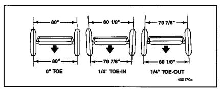
Figure 63 — Toe Measurements
