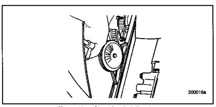
Figure 10 — Checking Belt Tension
