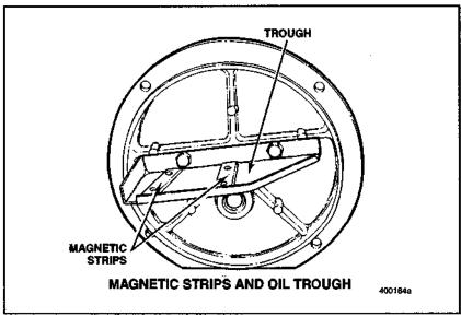
Figure 43 — Magnetic Strips and Oil Trough
