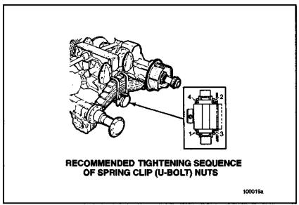
Figure 57 — Recommended Spring Clip Nut Tightening Sequence
