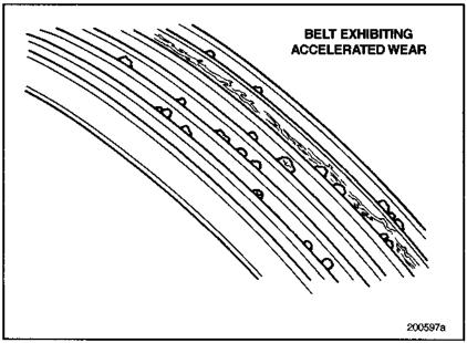
Figure 15 — Belt Exhibiting Accelerated Wear
