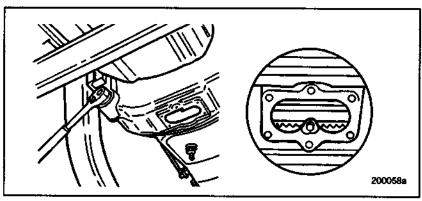
Figure 88 — Flywheel Timing Indicator
