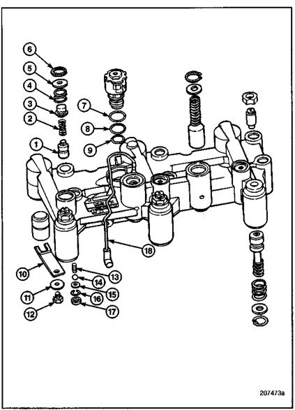
Figure 94 -- J-Tech Engine Brake Tune-Up Kit
