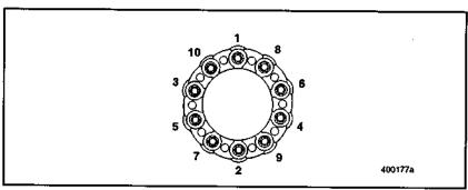
Figure 71 — Wheel Nut Tightening Sequence with Chain Clearance Spacers
