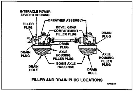
Figure 42 — Filler and Drain Plug Locations
