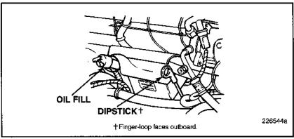
Figure 33 — Conventional Cabs Oil Fill and Dipstick Location
