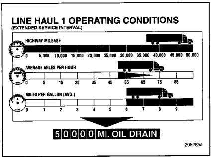
Figure 4 — Line Haul 1 Operating Conditions
