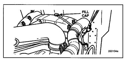
On LE and MR models, add the SCA packets into the pressurized surge tank which is located behind the cab on the left-hand side of the chassis, mounted above the air cleaner. (Refer to the illustration below:)
