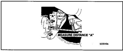
Figure 73 — Brakes Released Measurement
