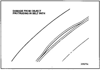
Figure 16 — Damage from Object Protruding in Belt Path
