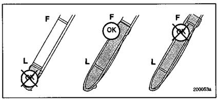
Figure 32 — Dipstick Oil Level Check
