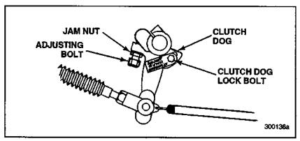
Figure 85 — Clutch Linkage
