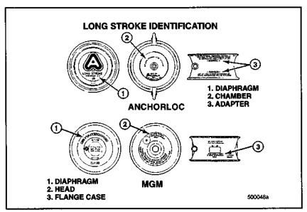
Figure 72 — Long Stroke Identification
