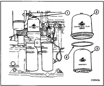
Figure 35 — Centri-Max® PLUS Oil Filter
