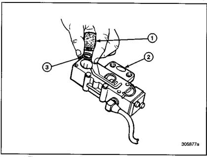
Figure 38 — Range Shift Valve Cover Spring and Fitter
