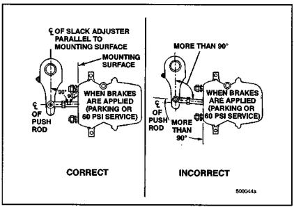
Figure 76 -- Proper Slack Adjustment
