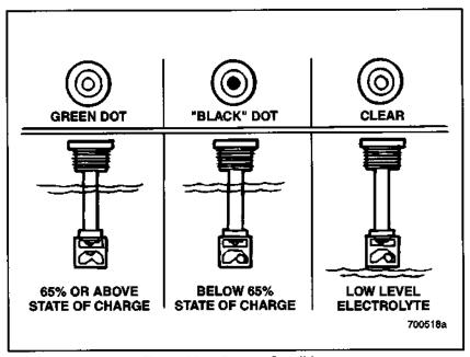
Figure 30 — Battery Condition
