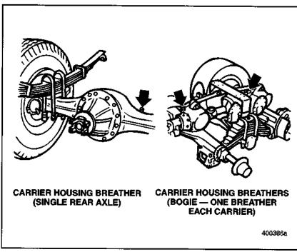
Figure 44 — Carrier Housing Breathers
