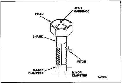
Figure 8 — Fastener Identification
