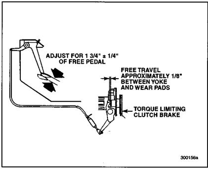
Figure 80 — Clutch Pedal Free Travel
