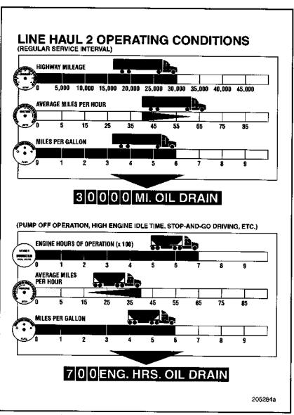
Figure 5 — Line Haul 2 Operating Conditions
