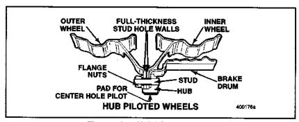
Figure 70 — Hub Piloted Wheels
