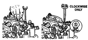
ADJUSTING SCREW SLOT MOVEMENT
