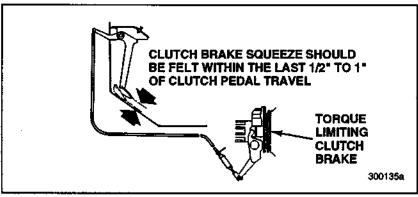
Figure 82 — Clutch Brake Squeeze — Spicer Easy Pedal
