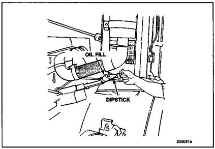
Figure 34 — Cab Forward Chassis Oil Fill and Dipstick Location
