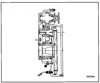
Figure 40 — REPTO Drain Plug Location
