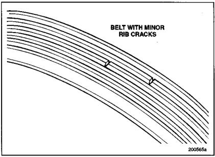
Figure 12 — Belt with Minor Rib Cracks
