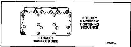
Figure 87 — Capscrew Tightening Sequence
