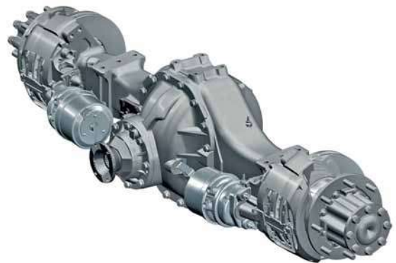
Rear axle, ring gear 410, hypoid, 10,8 t (771.003)
