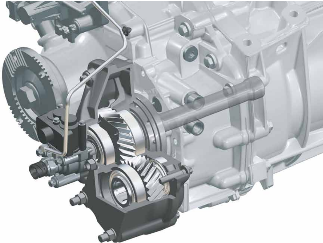
Power take-off NA MB 131-2c, pump (N2E) on transmission G 141-9
