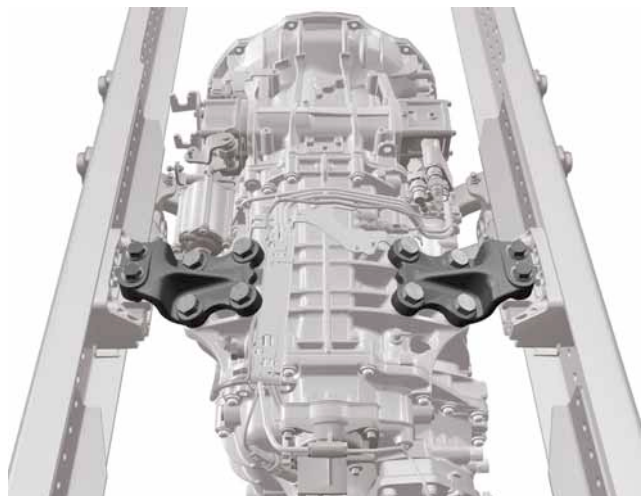
Transmission with bolted support arms
