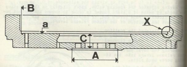
If there are some scratches on the "a" bearing surface, it has to be nely re-turned within the allowable surface fineness range of Ra = 1 3.2 micromillimetres.
