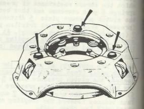
Carefully inspect and duly clean the separate parts of the clutch assembly and replace all defective or damaged parts by new ones.
