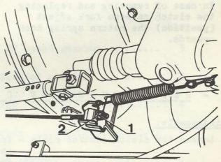
Otherwise readjust the spacing correctly as specified by means of the adjusting nut 2 and lock it properly by means of the lock nut 1. Then hook on the disconnected return spring again.
