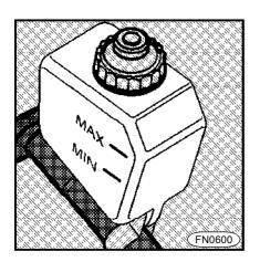
**n** The clutch is actuated hydraulically and completed with the air booster.
