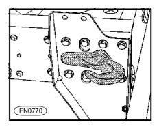
A special hook to hold the rope for the vehicle recovery is welded to the frame.
