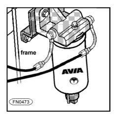
Unscrew drain bolts on the fuel filter bottom to allow draining of water from the fuel filter. When all dirt particles drip out, screw the bolts again.
