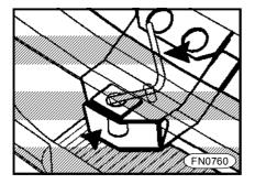
n Use the pin to attach the towing bar in the middle part of the front bumper. n When towing the vehicle with the engine at standstill and no gear speed shifted in gearbox, disconnect the propeller shaft not to damage the gearbox due to insufficient lubrication and release the spring-loaded cylinder in accordance with Chapter "Parking brake".
