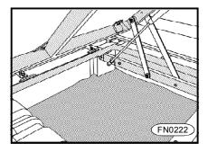
The storage compartment is accessible after unlocking the rubber element and tilting the couch.
