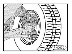
**n** If you notice that tire treads wear unevenly on the front axle, check and/ or have the front axle geometry adjusted at the authorized service station.
