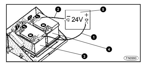
**n** The vehicle with a discharged battery may be started only by connecting it to the battery of some other vehicle with the same nominal voltage.
