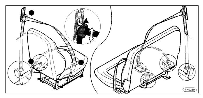
**n** The cabin is equipped with threepoint seat belts and retractors on two side seats. **n** The middle seat has got the twopoint seat belt and mechanical adjusting equipment.
