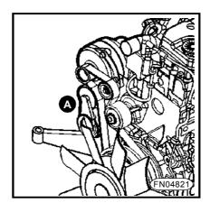
**n** The belt is tensioned automatically by the pulley (item A), which cares of the constant tension.
