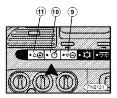
n The cruise control allows you to maintain a desired speed (engine speed - both on the move and in the PTO regime) - without actuating the accelerator pedal.
