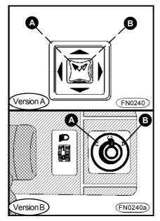
**n** Turn the controller to select adjustment of the left or right mirror.
