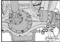
**n** Check the oil level and change the oil in axle final drive housings during service inspections.
