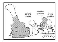
**n** The parking brake is of spring-loaded type and acts on wheels of the rear axle.
