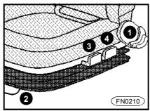
**n** The seat should be adjusted so that the driver could control the pedals safely.
