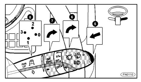
Position 2 - move the controller away from you and up - the engine brake works when the accelerator pedal is released (in the speed zone above the idle run).
