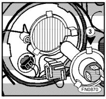
**n** Remove the faulty bulb and fit a new bulb - lugs (item 3) on the bulb base must engage into recesses of the headlamp.
