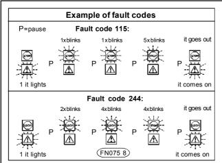
The indicator light "engine-stop" displays the fault code number. The example of fault code determination is illustrated.
