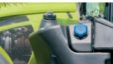
700 I fuel tank with integral 60 I urea tank
