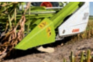
AUTO CONTOUR, ground pressure control with lateral leveling
