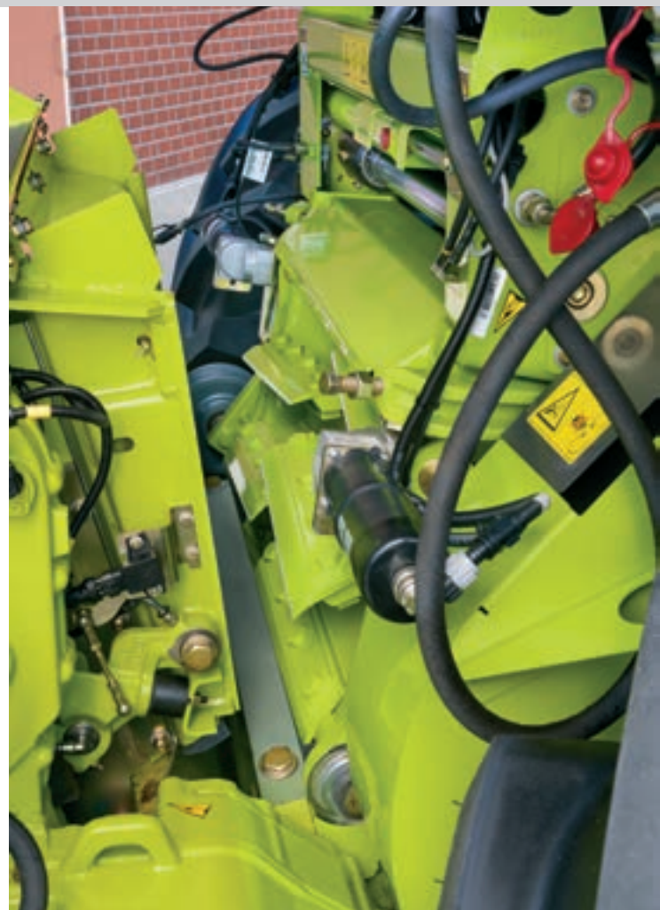
Ease of access to knife drum
