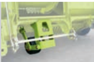
Support wheel for optimal ground-contour following
