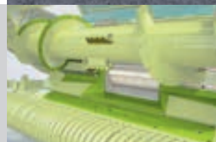
Support wheel for optimal ground-contour following
