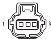
MANIFOLD ABSOLUTE PRESSURE SENSOR (8.0L)
