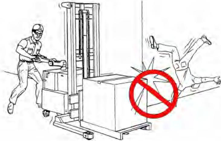
Observe applicable traffic regulations. Yield right-of-way to pedestrians. Slow down and sound horn at cross aisles and wherever vision is obstructed.
